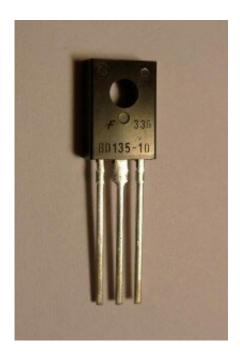
While the millions of transistors inside modern electronics are only micrometres in size, their function mirrors that of the familiar three-legged transistors of 1970s radios and home electronics kits. Credit: FLEET
