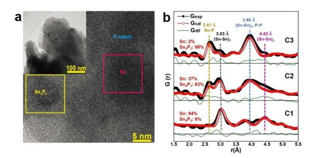
(a) Composite of  $Sn/Sn_4P_3$  nanodomains embedded in amorphous P matrix. (b) Quantitative analysis by PDF. Credit: Haijun Yu, Beijing University of Technology
