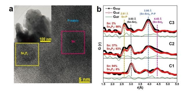
(a) Composite of Sn/Sn<sub>4</sub>P<sub>3</sub> nanodomains embedded in amorphous P matrix. (b) Quantitative analysis by PDF. Credit: Haijun Yu, Beijing University of Technology
