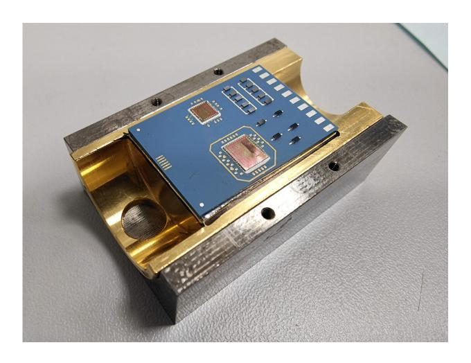
Picture 1: Ceramic circuit board with integrated cir-cuits resistant to high temperatures. Credit: Fraunhofer IZM
