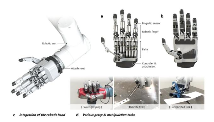
Fig. 1: Overview of the ILDA. a Configuration of the ILDA hand composed of five robotic fingers with fingertip sensors, the palm side integrating the actuators, and the controller and attachment. b ILDA hand with covers. c Ease of attachment of the ILDA hand to a developed robotic arm. d Actions performed using the ILDA hand such as grasping and manipulating everyday life tools, showing delicate and strong grasping. Credit: DOI: 10.1038/s41467-021-27261-0
