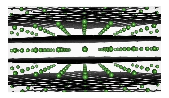
This illustration shows intercalation of lithium ions (green) in a graphite anode. Credit: Argonne National Laboratory
