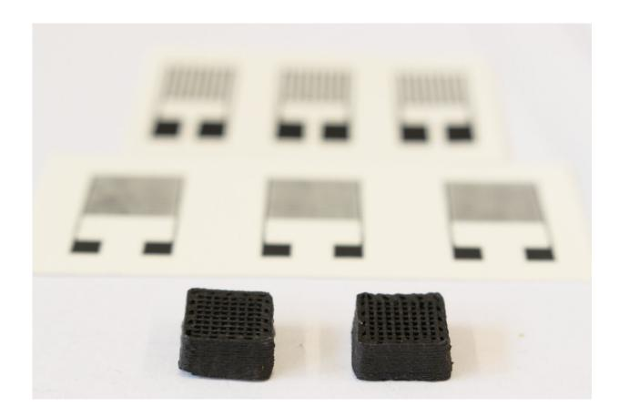
Novel material for printed circuits: Two test cuboids one centimeter wide from the 3D printer. The printed electronic sensors can be seen in the background. Credit: Empa
