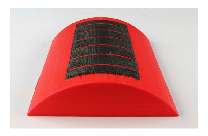
Non conformal printing: The flexible shellac ink could also be used on shapes such as PET bottles. Credit: Empa
