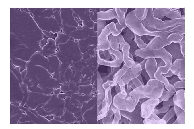
Scientists at the University of Texas at Austin have developed a new sodium metal anode for rechargeable batteries (left) that resists the formation of dendrites, a common problem with standard sodium metal anodes (right) that can lead to shorting and fires. Images were taken with a scanning electron microscope. Credit: Yixian Wang/University of Texas at Austin.
