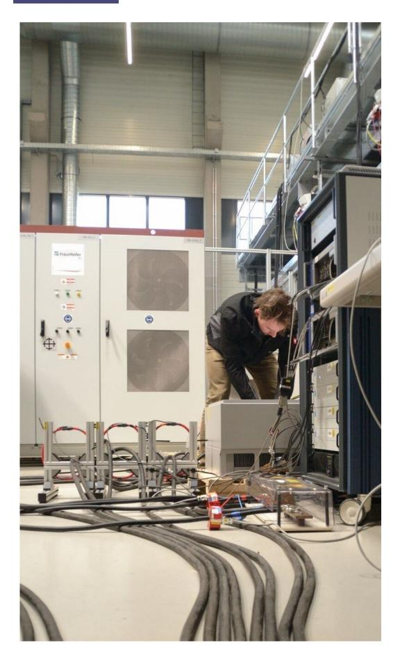
For the measurement-related proof of the grid-forming properties of converters, the power grid was simulated under laboratory conditions. Credit: Fraunhofer-Gesellschaft
