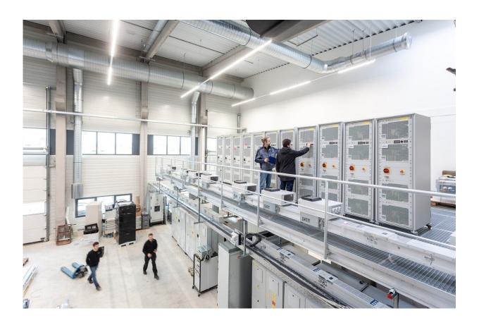
The Multi-Megawatt Lab at Fraunhofer ISE in Freiburg makes it possible to achieve highly precise characterization of the electrical proper-ties of converters up to a power of 10 MW. Credit: Fraunhofer-Gesellschaft
