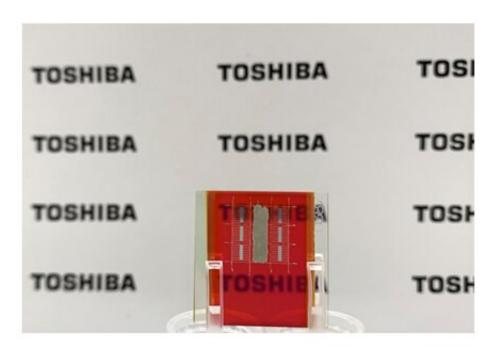
Figure 1: Toshiba's transparent  $Cu_2O$  solar cell. Credit: Toshiba Corporation News Releases
