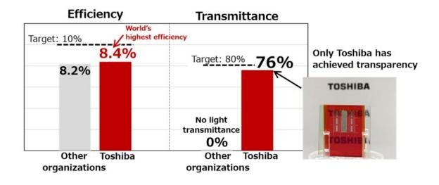
Figure 4: Transparent Cu2O cell development progress. Credit: Toshiba Corporation News Releases
