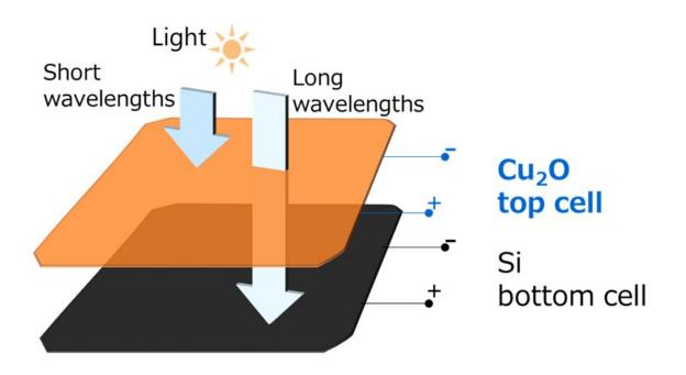
Figure 3: Schematic diagram of Cu2O-Si tandem solar cell. Credit: Toshiba Corporation News Releases
