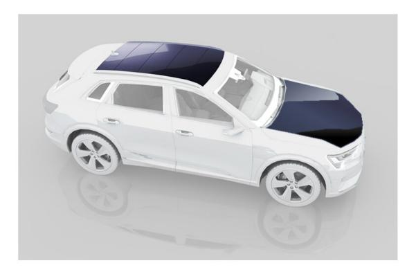
Figure 2: Image of a  $Cu_2O$ -Si tandem solar cell array installed on an EV. Credit: Toshiba Corporation News Releases
