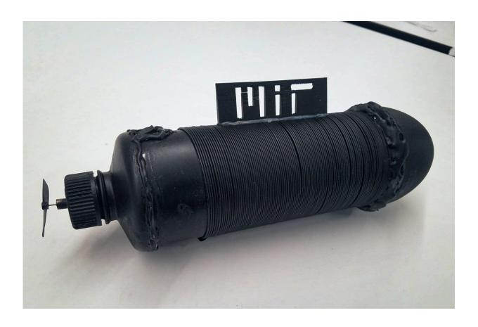
This submarine drone is powered by a 20-meter-long fiber battery that is wrapped on its surface. Credit: Tural Khudiyev, Jung Tae Lee, Benjamin Grena, Yoel Fink et al
