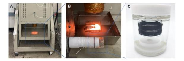
Photographs of synthesis process of DWNTY. (A) Vertical furnace, (B) winding process, and (C) as-produced DWNTY wound on a roll. Credit: *Science Advances*, DOI: 10.1126/sciadv.abl8631
