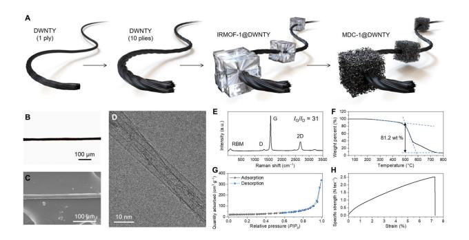
Basic properties of DWNTY. (A) Schematics illustrating the fabrication method to prepare MDC-1@DWNTY, (B) optical microscopy (OM) image, (C) scanning electron microscopy (SEM) image, (D) transmission electron microscopy (TEM) image, (E) Raman spectrum, radial breathing mode (RBM), (F) thermogravimetric analysis (TGA), (G) N2 sorption isotherm, and (H) stress-strain curve of DWNTY. a.u., arbitrary units; wt %, weight %. Credit: *Science Advances*, DOI: 10.1126/sciadv.abl8631
