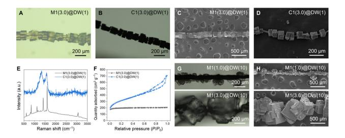
Characterization of IRMOF-1@DWNTY and MDC-1@DWNTY. (A and B) OM images, (C and D) SEM images, (E) Raman spectra, and (F) N2 sorption isotherms of M1(3.0)@DW(1) and C1(3.0)@DW(1). (G) OM images and (H) SEM images of M1@DW(10) at different precursor concentrations. Credit: *Science Advances*, DOI: 10.1126/sciadv.abl8631
