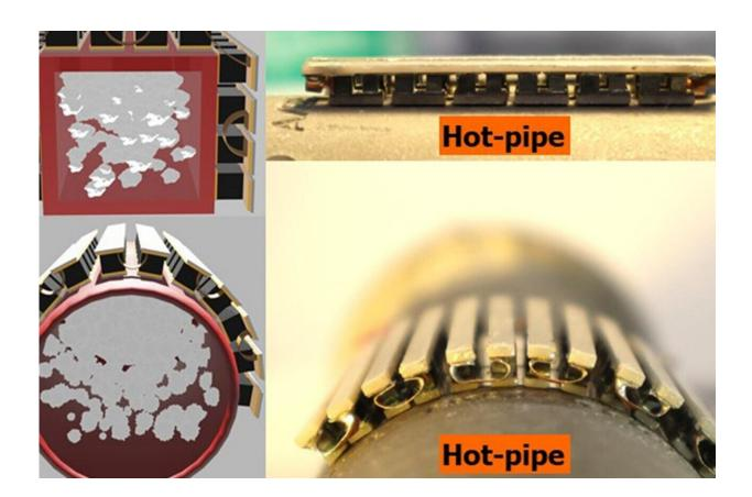
A new flexible thermoelectric device can wrap around pipes and other hot surfaces and convert wasted heat into electricity. Credit: Penn State
