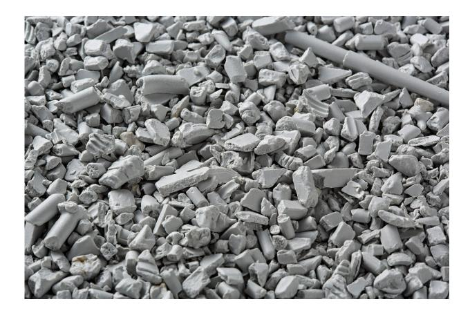
Plastic granulate from recycled plastic. Credit: Fraunhofer LBF/Ursula Raapke
