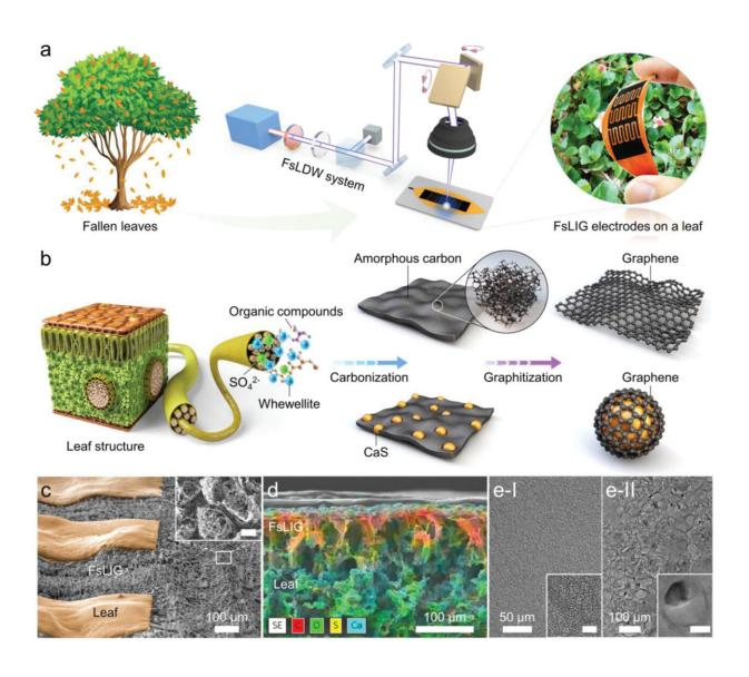
The schematic illustration of the production of femtosecond laser-induced graphene. Credit: Korea Advanced Institute of Science and Technology)
