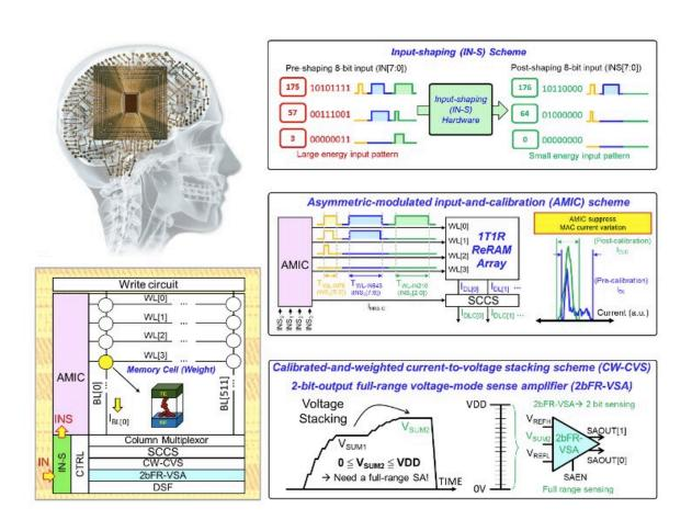
Die photo and macro structure along with the proposed scheme (input-shaping scheme, asymmetric-modulated input-and-calibration scheme, calibrated-and-weighted current-to-voltage stacking scheme, and 2-bit-output full-range voltage-mode sense amplifier). Credit: Hung et al.
