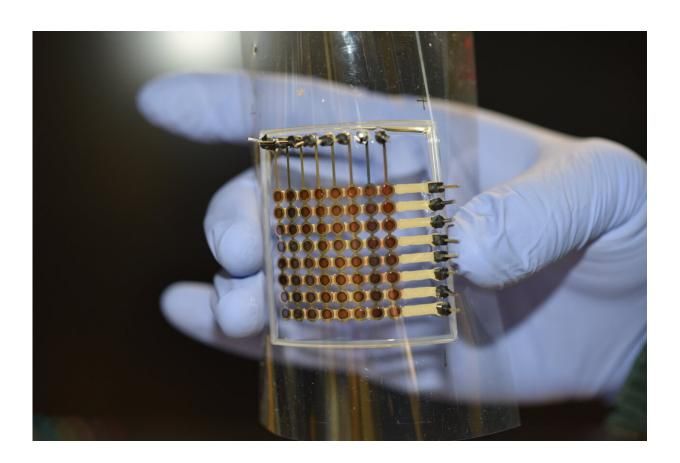
The fully 3D-printed flexible organic light-emitting diode (OLED) display prototype is about 1.5 inches on each side and has 64 pixels. Every pixel works and displays light. The 3D-printed display is also flexible, which could make it useful for a wide variety of applications, such as foldable smartphone displays. Credit: McAlpine Group, University of Minnesota
