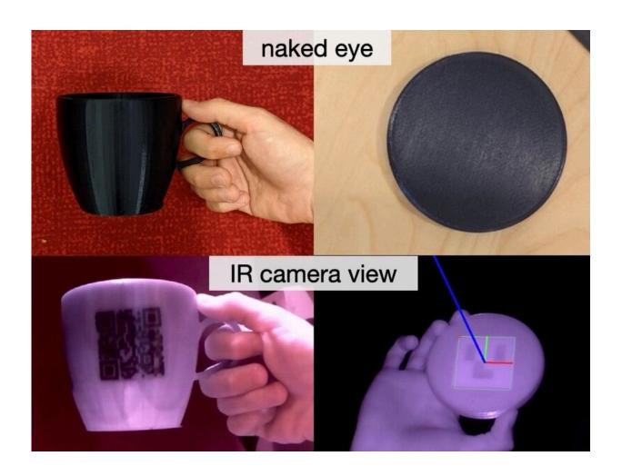
MIT scientists built a user interface that facilitates the integration of common tags (QR codes or ArUco markers used for augmented reality) with the object geometry to make them 3D printable as InfraredTags. Credit: MIT CSAIL
