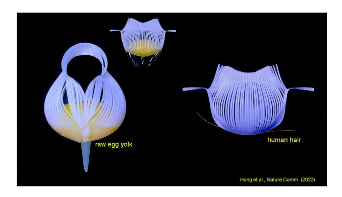
Engineering researchers from North Carolina State University have demonstrated a new type of flexible, robotic grippers that are able to lift delicate egg yolks without breaking them, and that are precise enough to lift a human hair. Credit: Jie Yin, North Carolina State University
