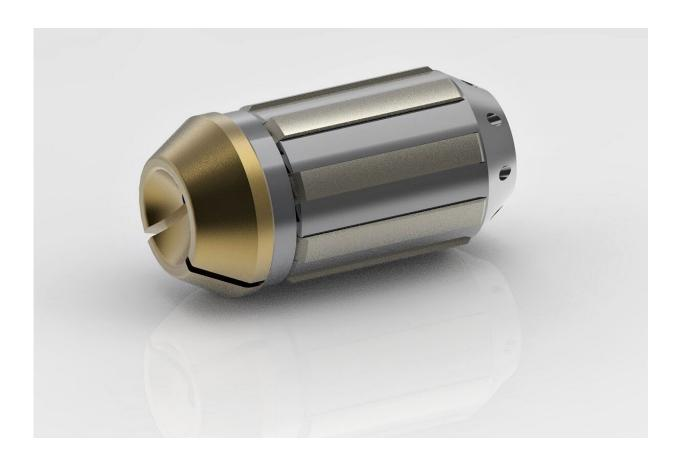
The micro drilling turbine with a diamond drill bit is only 10 centimeters long and has a diameter of 3.6 centimeters. When drilling, it rotates at up to 80,000 revolutions per minute. Credit: Fraunhofer-Gesellschaft
