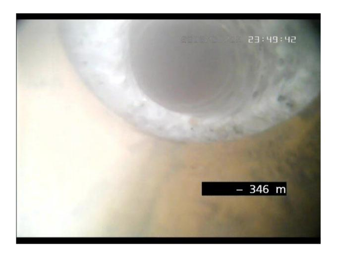
View of a freshly drilled side arm at 346 meters. The micro drilling turbine milled out the granite rock cleanly. Credit: Fraunhofer-Gesellschaft
