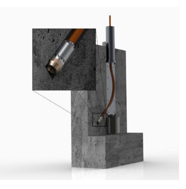
Simple and reliable: the sheet steel deflection shoe guides the drilling tool outward at an angle of 45 degrees. Credit: Fraunhofer-Gesellschaft
