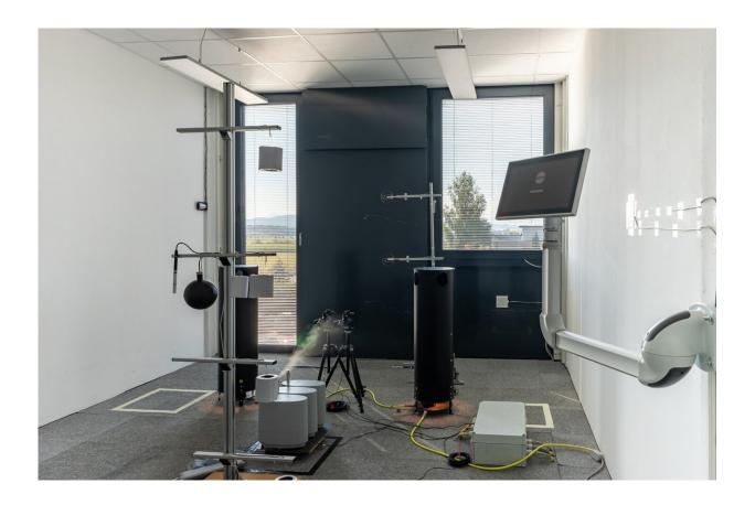
View of the test room behind the modular facade containing measuring instruments. Credit: Fraunhofer-Gesellschaft
