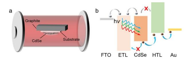
(a) Schematic diagram of RTE. (b) Schematic diagram of CdSe solar cells design based on bandgap engineering. Credit: Higher Education Press Limited Company
