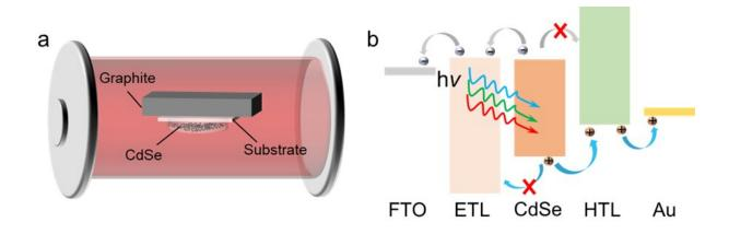
(a) Schematic diagram of RTE. (b) Schematic diagram of CdSe solar cells design based on bandgap engineering. Credit: Higher Education Press Limited Company
