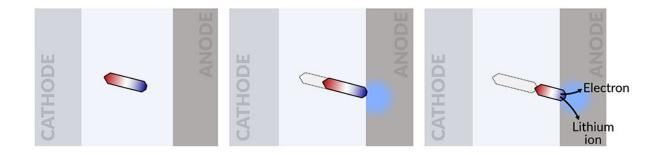
When an island of inactivated lithium metal travels to a battery's anode, or negative electrode, and reconnects, it comes back to life, contributing electrons to the battery's current flow and lithium ions for storing charge until it's needed. The island moves by adding lithium metal at one end (blue) and dissolving it at the other end (red). Researchers from SLAC and Stanford discovered that they
