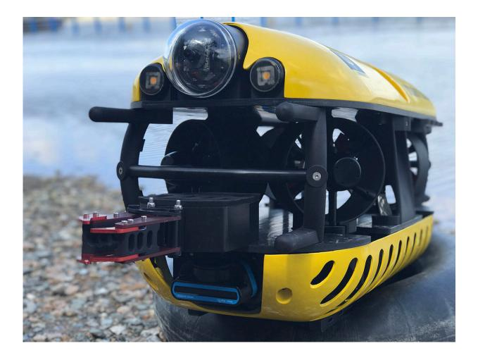
SeaClear's ROV TORTUGA is known as 'the cleaner' robot. It collects the litter from the seafloor. Credit: SeaClear, 2021
