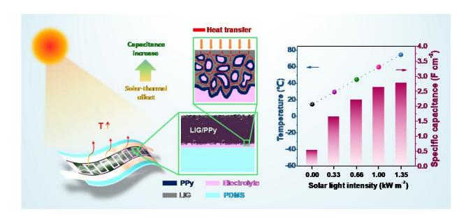
Schematic diagram of fabricating process for the solar-thermal microsupercapacitor and their energy storage performance under different light intensities. Credit: Li Nian
