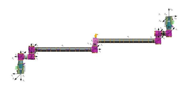
In the research, the simulation results of our recursive composite adaptive control algorithm are presented in comparison with the direct adaptive control algorithm. The coordinate frames of the manipulator of the Chinese Space Station are plotted here. Credit: Space: Science & Technology
