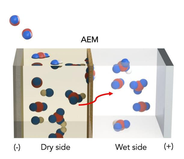
Illustration of a carbon capture process designed by UIC College of Engineering scientists. Carbon dioxide from air or flue gas is absorbed by a dry organic
