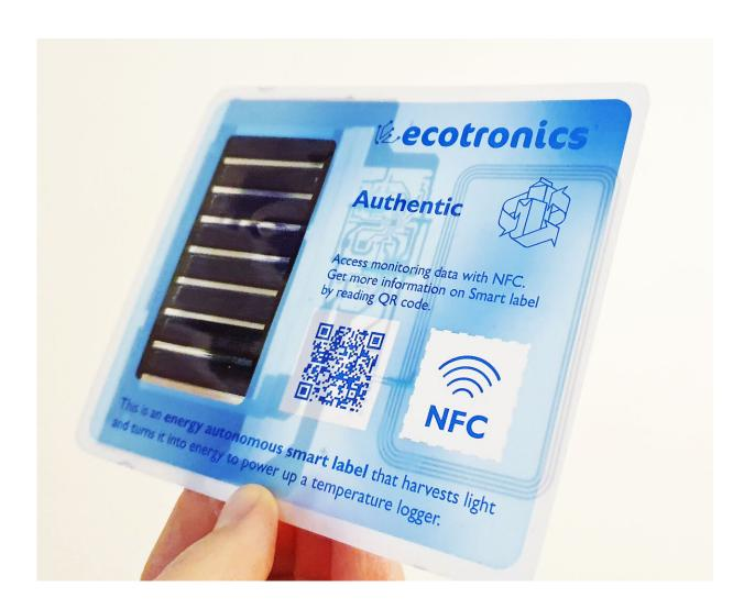
VTT and university partners have integrated a thin and flexible electronic label for condition monitoring based on bio-based and environmentally friendly materials, sustainable manufacturing processes, and eco-design. The energy is harvested from light. Credit: VTT Technical Research Centre of Finland
