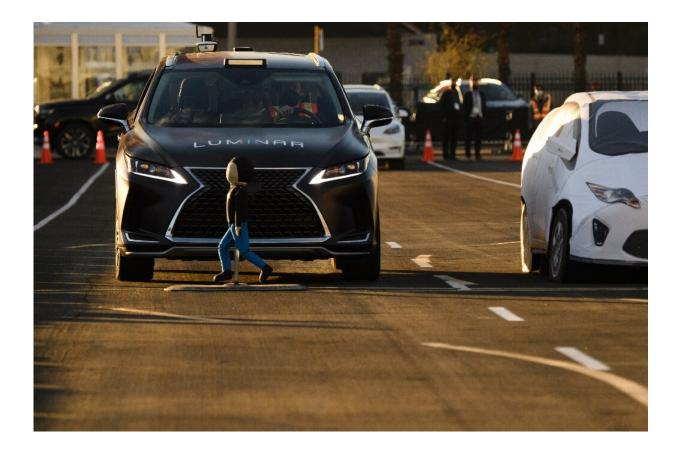
A vehicle with Luminar's lidar-based Proactive Safety pre-collision braking crash avoidance sensors stops to avoid a child-sized test dummy at the Consumer Electronics Show in Las Vegas.
