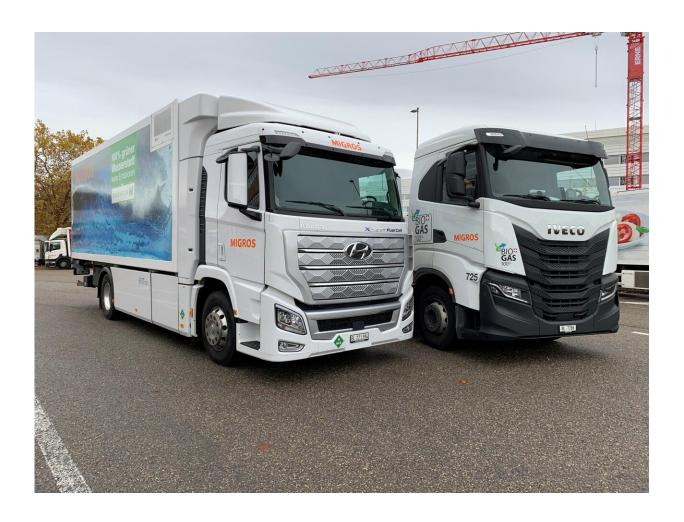
Alternative powertrain systems reduce greenhouse gas emissions in freight transports: Migros operates hydrogen and biogas trucks. Credit: Migros
