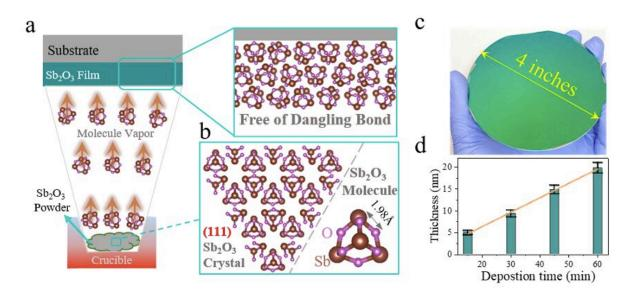
Fig. 1: Fabrication of a wafer-scale Sb2O3 film via STED. a, the schematic figure of thermal evaporation process to fabricate vdW dielectric film. b, the crystal structure of Sb2O3. C, the Sb2O3 film of 4 inches that we fabricate. d, the precise control over the film thickness. Credit: DOI: 10.1038/s41928-021-00683-w
