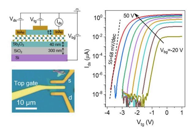
The schematic figure and optical image of MoS2 FET that are gated with Sb2O3 film as dielectrics, as well as its transfer characteristic curves of the FET. Credit: Zhai et al.
