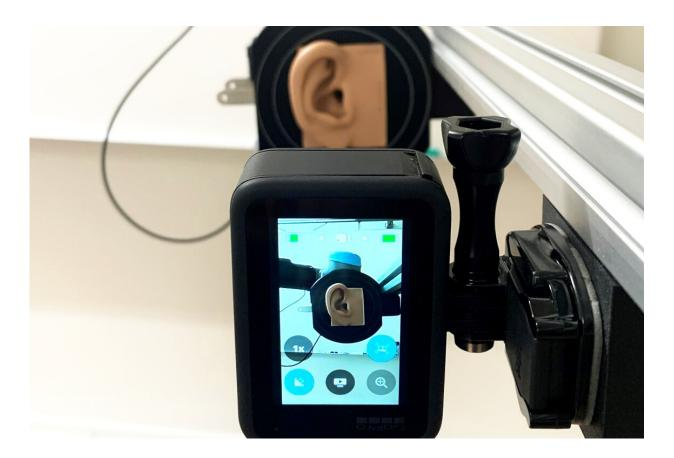
An artificial ear packed with sensors and a robot will test the earbuds. Credit: SINTEF
