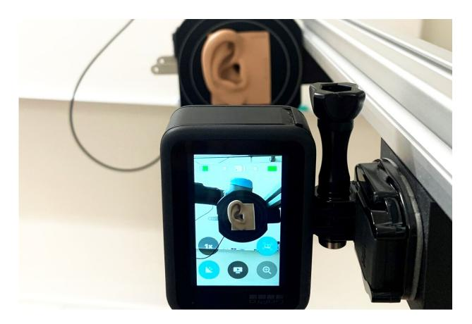
An artificial ear packed with sensors and a robot will test the earbuds. Credit: SINTEF
