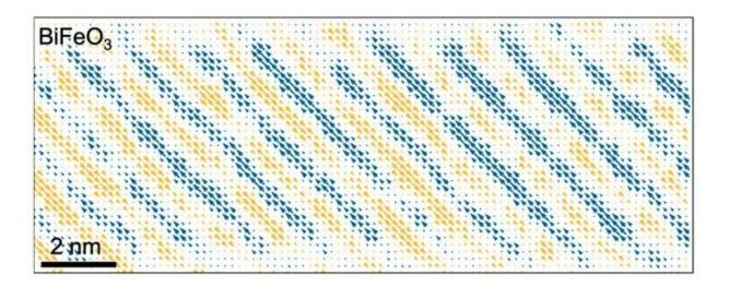
This image shows the alternating electrical dipoles in a newly formed antiferroelectric that was created by stacking layers of bismuth ferrite with other insulators. Credit: Mundy et al, *Science Advances*
