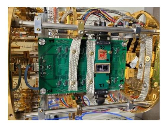
Green commercial circuit boards—the largest is 11.4 cm (4.5 in) by 19 cm (7.5 in)—inside a dilution refrigerator. When enclosed and pumped down, the system reaches temperatures only a few thousandths of a degree above absolute zero. Credit: NIST
