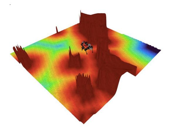
A Signed Distance Field (SDF) computed from the local map around the robot was used to generate repulsion forces to stay away from obstacles, especially in narrow corridors. Red means closer to obstacles and blue farther away. Credit: Mattamala, Chebrolu & Fallon.
