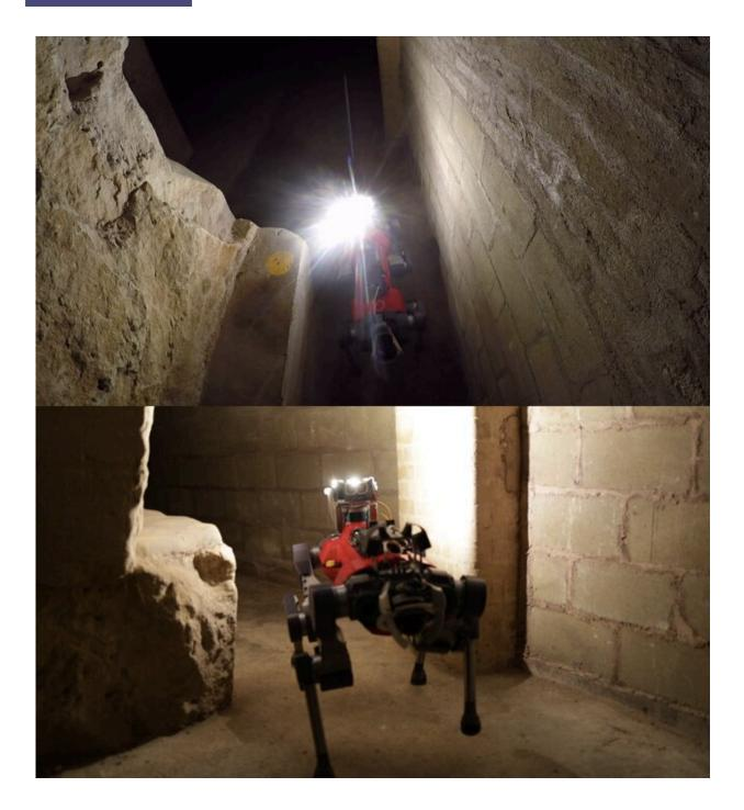
The team's experiment in a decommissioned mine near Wiltshire, UK, was a 60 m long path. The robot traversed it without collisions, despite the challenging lighting conditions and narrow passages. Credit: Mattamala, Chebrolu & Fallon. Picture by Oliver Barlett.
