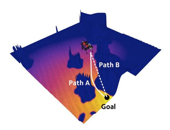
The Geodesic Distance Field (GDF) was used to determine directions (a
