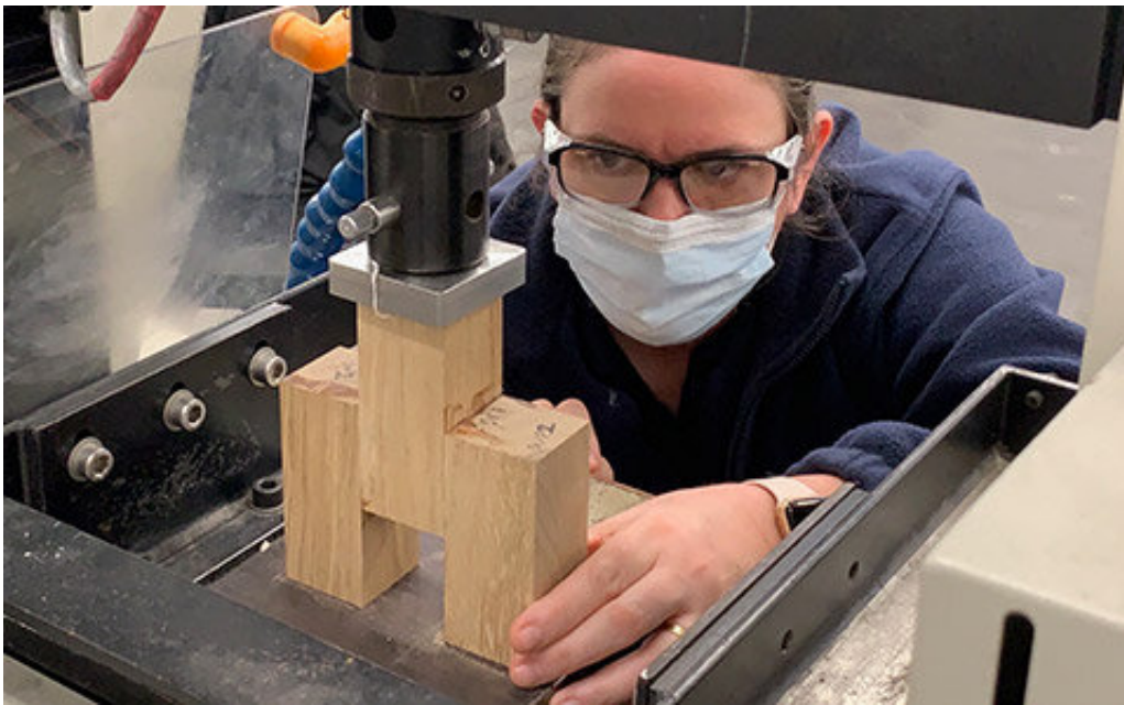
Dr Nicola Symonds setting up a shear test on a glue sample. Credit: University of Southampton
