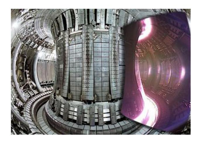
Internal view of the JET tokamak. Credit: EFDA-JET/wikipedia, CC BY-SA
