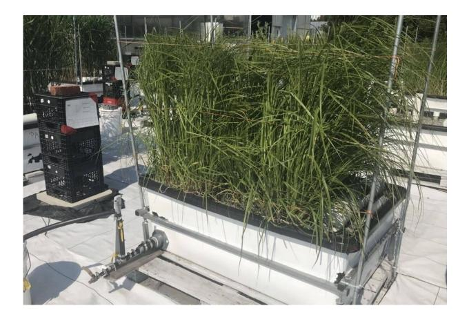
Mesocosm experiment for pesticide removal in filter marshes. Credit: University of Montreal
