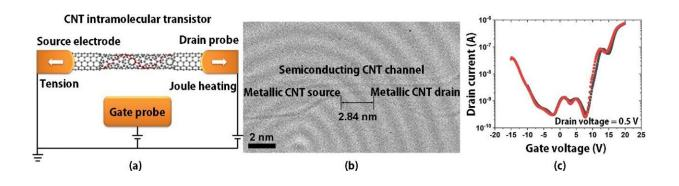
(a) Schematic diagram and (b) a transmission electron microscopy image of a CNT intramolecular transistor. (c) Current–voltage characteristics of the transistor. Credit: Daiming Tang National Institute for Materials Science
