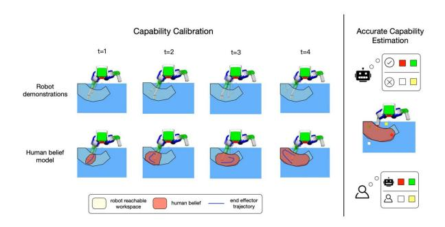
The robot models human belief update and uses expressive motions to show its reachable workspace. After the calibration, the human with accurate capability estimation can assign proper roles to the robot. Credit: Gao et al.
