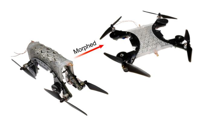
Drone able to morph and bends using liquid metal. Credit: Virginia Tech
