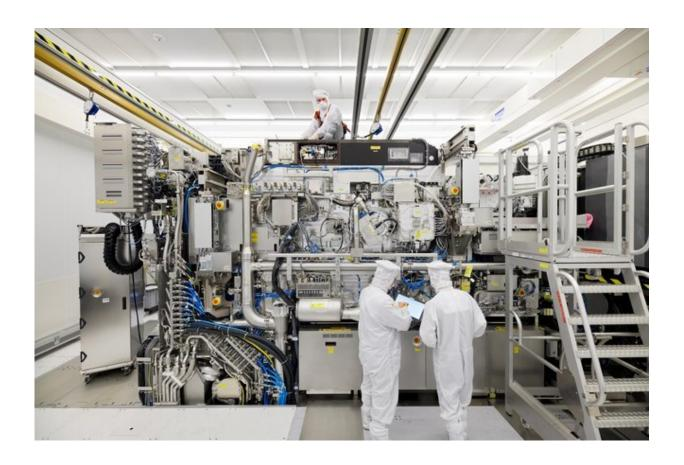
An EUV lithography machine from the company ASML is being assembled. Credit: Bart van Overbeeke
