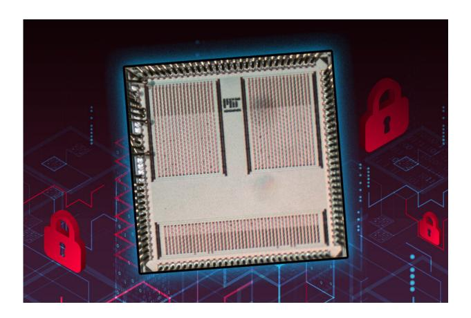
MIT researchers developed an application-specific integrated circuit (ASIC) chip, pictured here, that can be implemented on an internet of things device to defend against power-based side-channel attacks. Credit: Massachusetts Institute of Technology
