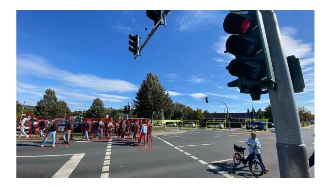
The KI4PED project focuses on pedestrians rather than vehicles. People are detected and tracked using LiDAR sensor data and AI. Credit: Fraunhofer-Gesellschaft
