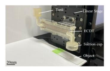
Researchers from SIT, Japan, have recently developed an electrochemical reaction-based transducer that allows smooth control of fluidic systems in soft robots, enabling self-sensing actuation without complexity and opening doors to miniaturized soft robotic technology. Credit: Shingo Maeda from Shibaura Institute of Technology, Japan
