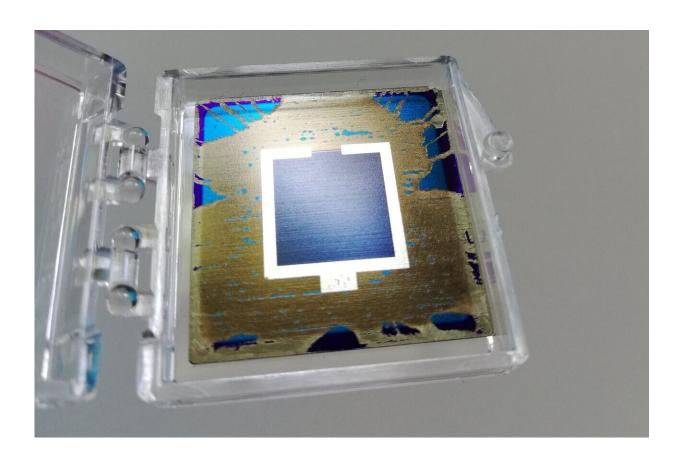
A standard silicon solar cell is combined with a perovskite top cell. This tandem solar cell could reach high efficiencies. Credit: Silvia Mariotti / HZB
