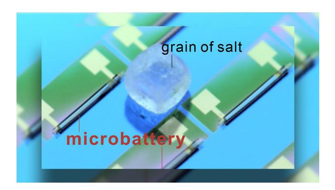
The world's smallest battery is smaller than a grain of salt and can be produced in large quantities on a wafer surface. Credit: TU Chemnitz/Leibniz IFW Dresden
