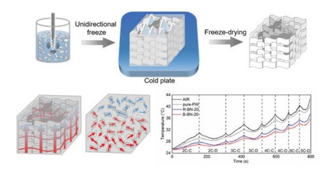
The process the researchers followed to enhance heat dissipation performance management in lithium ion batteries. Credit: Zhejiang University
