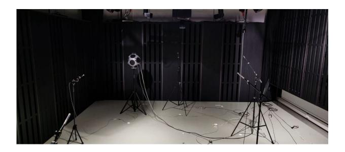
The walls of the Arni room have rotating panels. A spherical loudspeaker plays sound to all directions, and the acoustic properties can be measured with several microphones at the same time. Credit: Aalto University / Karolina Prawda
