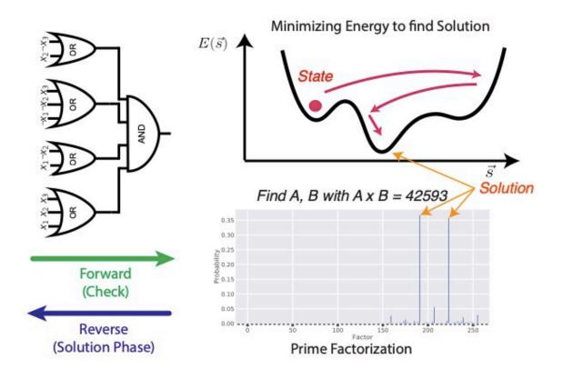
Left: Using digital logic to both do the forward (check) and reverse (solution) phase of computation. Top Right: The sampler probabilistically searches for the best solutions in the space. Bottom Right: An important application is solving factors for semi-primes, a problem at the heart of modern cryptography, and usually considered intractable. Credit: Patel, Canoza & Salahuddin.
