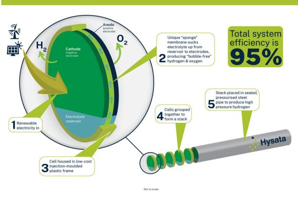
How Hysata's Capillary-Fed Electrolysis (CFE) cell works
